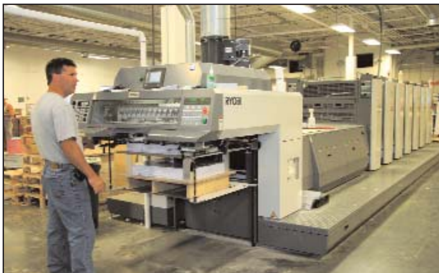
Pressman Jeff Osborne at the Ryobi 755 press which can print six colors at a time and has a coater.
